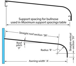
Span to be used in determining wind pressure capacities of bullnoses
